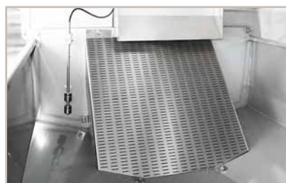
strainer on the pan outlet, level probe
